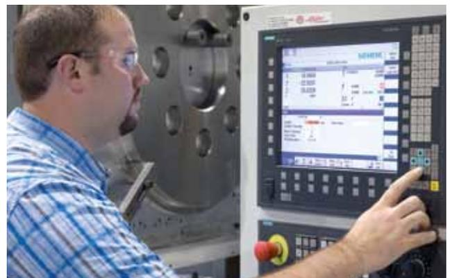
Programming as easy as 1-2-3: Using the SINUMERIK Operate interface, a machinist can turn on coolant flow by 1) pressing Cycle Stop to stop the machine, 2) Coolant On and 3) Restart.
