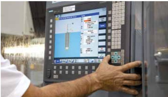
Central to MTM's retrofit program has been the Siemens SINUMERIK 840D sl control, which features the SINUMERIK Operate interface. The highly intuitive interface enables both programmers and operators to easily capitalize on the broad capabilities of the control.
