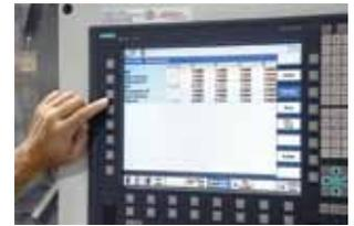
Work offsets for compound angles can be scaled and rotated using the Frames function of the Siemens SINUMERIK Operate interface. Many advanced machining operations can be managed simply, without the use of time-intensive manual G-code programming.
